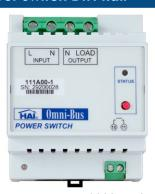
Control general purpose resistive: 3000W (13A)@230V~, motor: 4hp (3000W)@230V~, ballast (fluorescent lights): 3000W@230V~, low voltage transformer: 3000W@230V~. Designed for HAI's international markets using 220-240V~, 50Hz.
