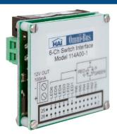
Connects up to six third-party switches to the Omni-Bus network. Six LED outputs control two-lead bi-color or single color LED indicators for each switch. Omni-Bus component designed for HAI's international markets using 220-240V~, 50Hz.
