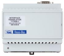
The "gateway" of the Omni-Bus system, this device allows HAI Controllers (OmniLT, Omni IIe, OmniPro II, Lumina, and Lumina Pro) to interface with an Omni-Bus network. Designed for HAI's international markets using 220-240V~, 50Hz.
