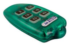
Wireless RF transmitter built into a convenient keyfob. Up to six channels available. Controls dimmer, power switch, relay, or inputs into HAI controller. Requires RF Transceiver (116A00-1).Designed for HAI's international markets using 220-240V~, 50Hz.
